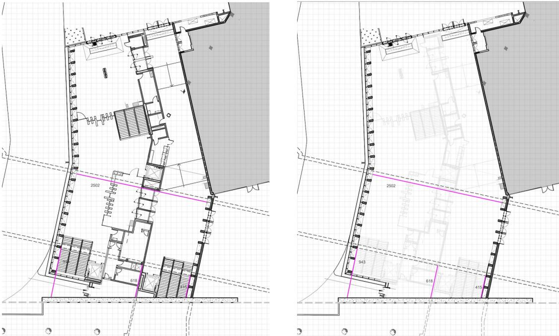
*Current plan vs current plan removing all the walls inside the proposed edicule.
