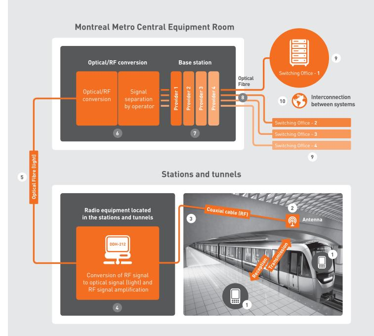
The mobile devices users in the Montreal Metro (1) are connected to the mobile service network by transmitting and receiving radiofrequency (RF) signals to and from antennas (2). These antennas are located through the Metro stations and tunnels.
