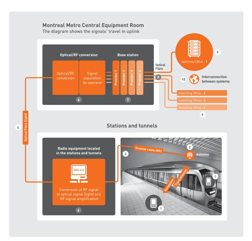
The mobile devices users in the Montreal Metro (1) are connected to the mobile service network by transmitting and receiving radiofrequency (RF) signals to and from antennas (2). These antennas are located through the Metro stations and tunnels.
